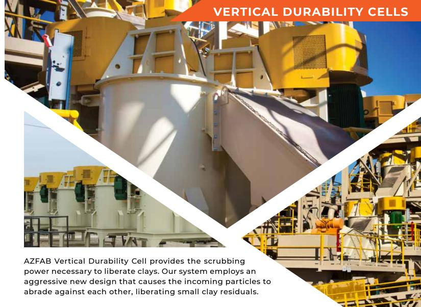
Paddles inside the Vertical Durability Cell provide the force to scrub the sand and liberate clay particles
